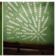
After the screen has been exposed, the print image, the printing stencil, is developed in the washout basin. The unexposed emulsion is washed from the fabric. The remaining screen fabric remains sealed. The screen is moistened with water on both sides, wiped over the entire surface with a sponge and then rinsed with normal water pressure. The printing stencil is prepared in the screen: printing (yellow, translucent) and non-printing (green, opaque) areas.
