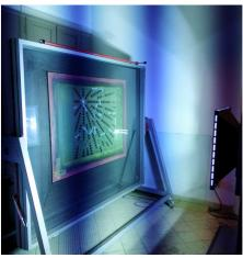
Exposure to ultraviolet light makes the emulsion that the light hits water and solvent resistant. The drawing on the film prevents exposure of the emulsion to the areas behind it. These unexposed areas are still water-soluble. The exposure time is set on the electronic exposure timer. The exposure time depends on the mesh fineness of the screens used (at least 45 seconds for 100 mesh, 1:20 min for 48 mesh, 1:40 min for 32 mesh).
