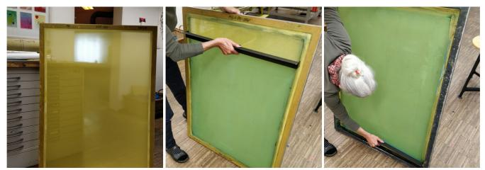
The screen fabrics are coated on both sides with the light-sensitive emulsion using a coating trough. Start with the print side. This is the side of the screen where the fabric is glued to the aluminium frame. When printing, the screen lies with this side down on the printing table. Then, by coating the squeegee side, the emulsion is pressed back into the mesh of the fabric. The squeegee side is the side on which the squeegee is used during printing, i.e. the ink is pressed through the fabric.
