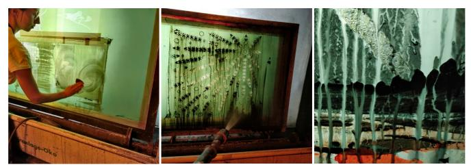
After printing, the screen is cleaned. The ink should be completely removed from the screen. To do this, the screen is wet from both sides, rubbed down with a sponge and detergent dissolved in water and rinsed off. In the case of inks that dry very quickly, the water pressure must be increased to avoid strong ghost images, which are coloured threads in the fabric. (Kärcher with minimum water pressure)
