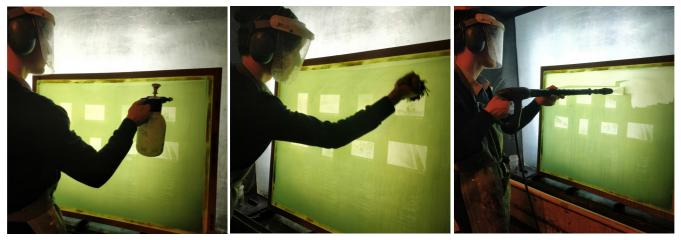
To remove the stencil, both sides of the screen fabric are sprayed with the de-coating chemical, which is then rubbed in with a thick, solvent-resistant brush. When the emulsion begins to dissolve, the fabric is sprayed freely from both sides with maximum increased water pressure (switch on the Kärcher, wear hearing protection). You start with the pressure side of the screen, i.e. the one on which the fabric is stretched. The clean, dry screens are then available for a new printing cycle.
