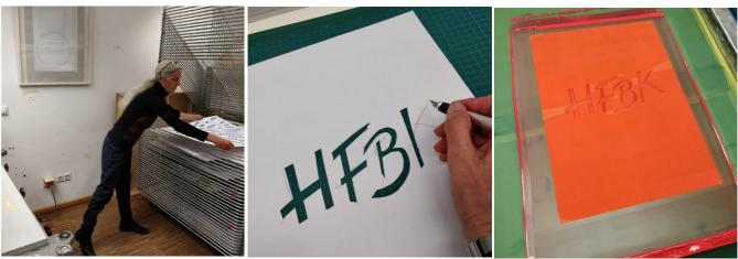
One way to print without an exposed screen is with paper masks. To do this, the areas that are to be printed are cut or torn from thin paper. This mask is placed in the correct position on the proof sheet. The masking paper blocks the way for the ink to reach the printing paper, which is why only what has been cut out is printed.
