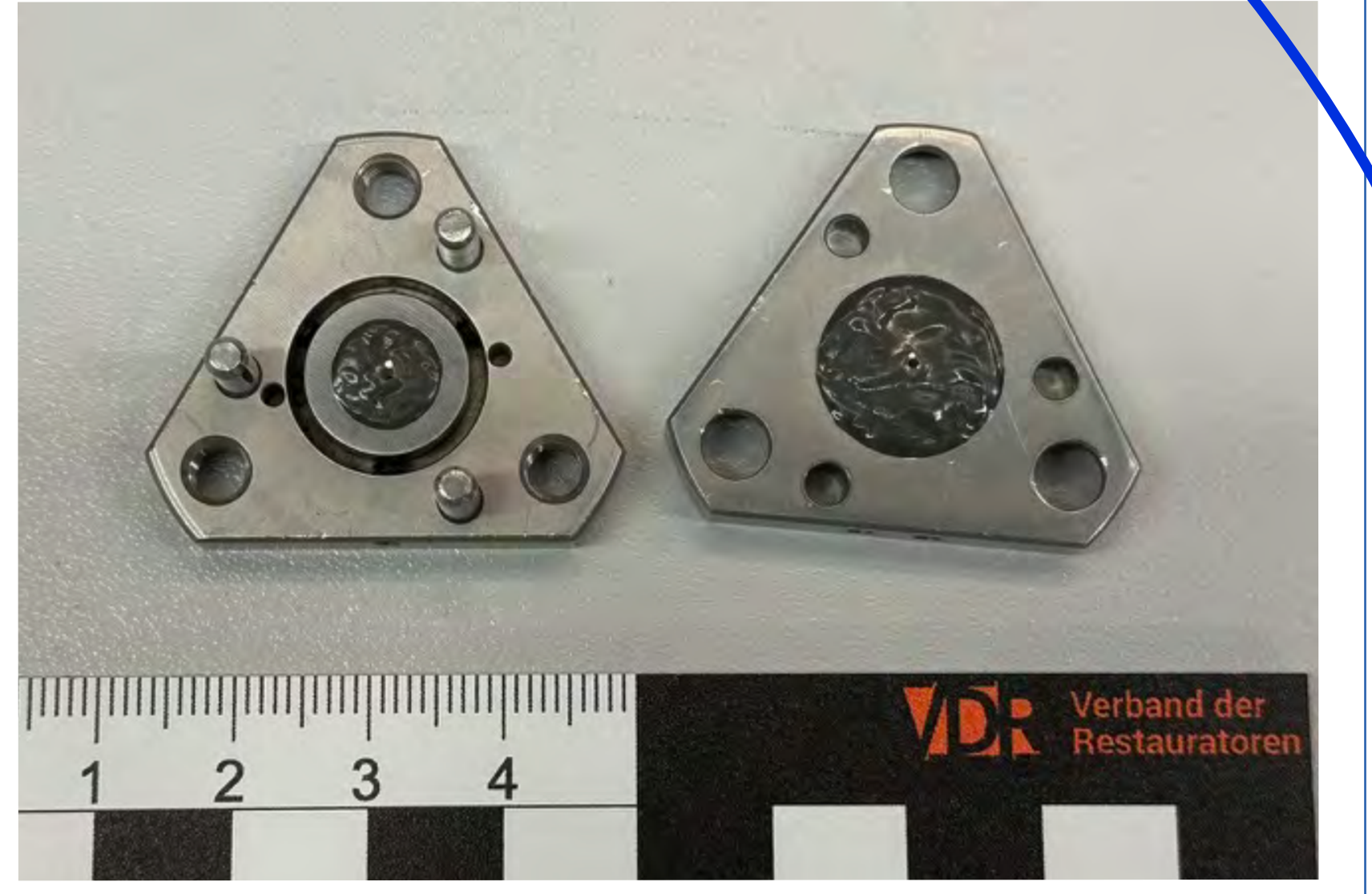
Fig. 7: Sampling for FTIR in transmission mode. Micro-sample is placed on the diamond and measured in transmission for binder, pigment and filler analysis. Credit: Zeynep Alp, 2025.
