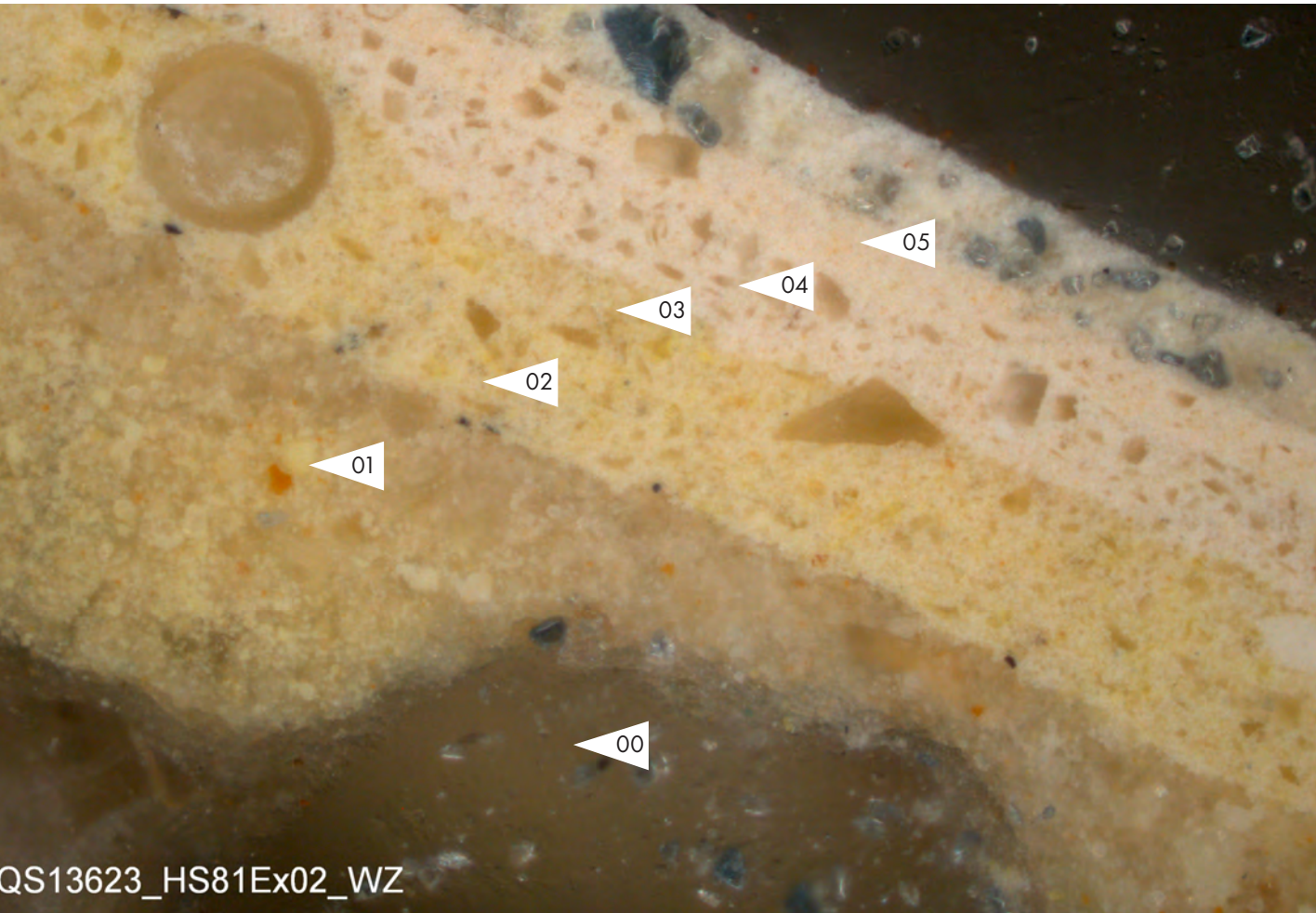
Fig. 4: Cross section made from the on-site sample, HS81Ex02 (Fig. 1), showing 5 paint layers under visible light microscope with 50x magnification. Credit: Zeynep Alp, 2024.
