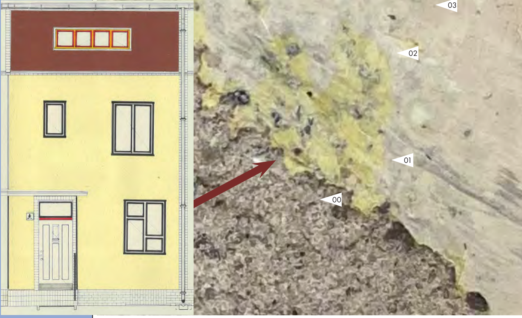
Fig. 1: Left: colour plan from the Brenne Architekten documentation (photo credit: Brenne Architekten). Right: Exposure from HS81Ex01 WZ, showing 3 paint layers (photo credit: Jana Hainbach).
